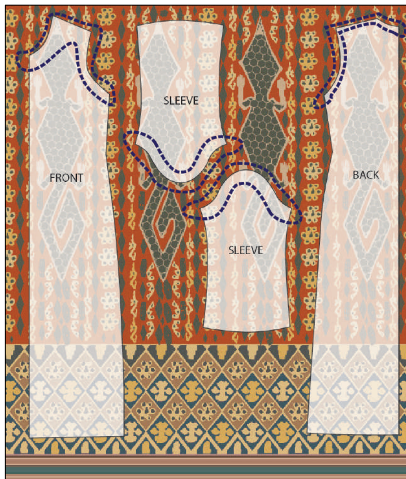
Figure 4. Technical drawing using regular pattern for Women clothes with Sumba Woven. Source: Ningsih, 2018
