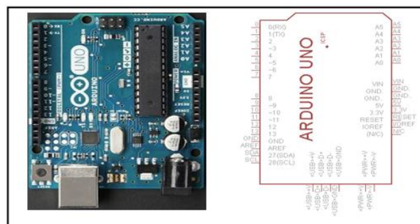
Gambar 6. Rangkaian Minimum Sistem Arduino Uno
