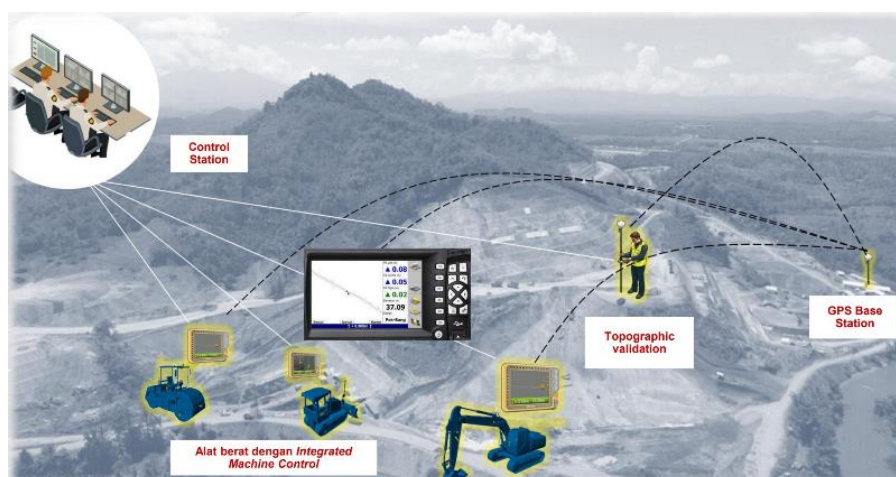
Gambar 2. Cara kerja 3D machine control (Position Indonesia, 2021)
