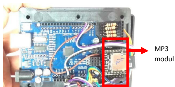
Fig. 10. MP3 player board installation
